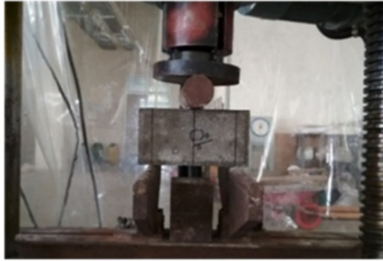
Fig. 7. Paving block under flexural loading.
