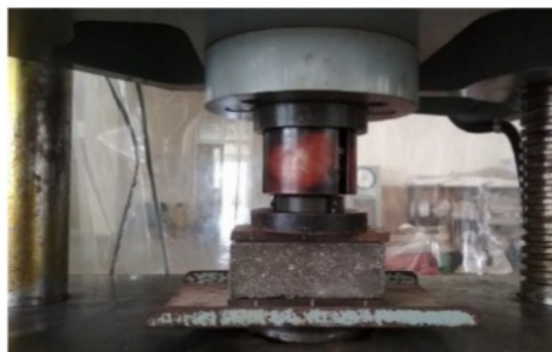
Fig. 6. Paving block under compression.
